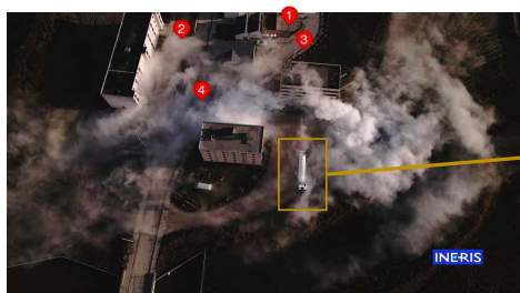
Top view photo of trial site. The numbered red pins indicate the positions of the sensors during the successive trial
