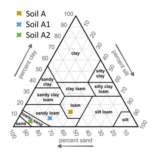
In order to test the influence of soil texture on soil water retention, sand content was artificially increased by supplementing the natural soil with washed quartz sand:
